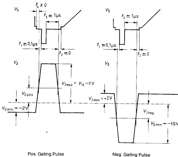
$$\begin{aligned} t_1 &\geq 0.5 \mu s \\ t_2 &\geq 0 \mu s \\ t_3 &\geq 2.5 \mu s \\ t_4 &\geq 0 \mu s \end{aligned}$$
